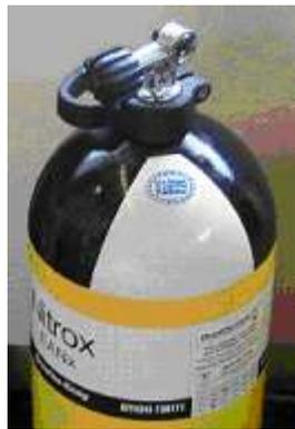
The Carriage of Dangerous Goods Regulations (1996) requires that cylinders are either correctly labelled with their contents OR that they are painted in the approved scheme (i.e. for compressed air and nitrox this means that black and white quarters are painted on the shoulder).
